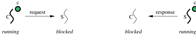
Figure 2. Synchronous communication between a client and a server in a component-based system. Left side: During the request the client thread C donates its timeslice c to the server thread S . Right side: When the server responds, the kernel returns the previously donated timeslice c back to the client.
